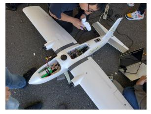
Last year's system was built from a commercial-off-the-shelf styrofoam airframe. From there, an ArduPilot-based autopilot module, camera, on-board image processing computer, radios, and landing gear were added to complete the vehicle itself. Air-to-ground communications were achieved using the MAVLink protocol, a Django web server, and a React client. Two TensorFlow-based computer vision models were trained to independently perform ground target detection and classification. Obstacle
